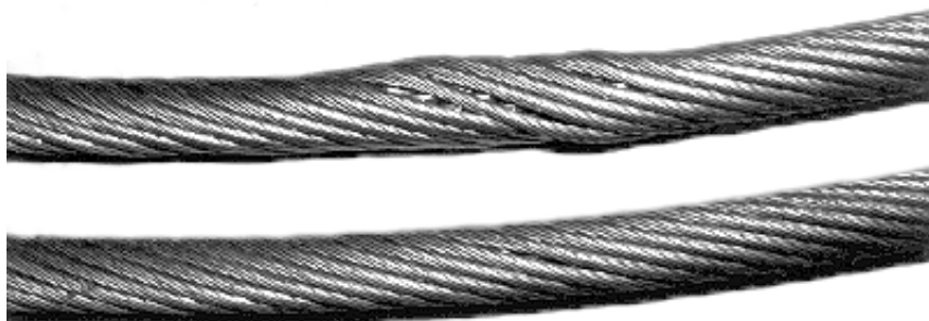
Drum crushing is one of the leading causes of early rope retirement. When installing a new rope, the foundation and all subsequent layers must be installed tightly and without gaps.
