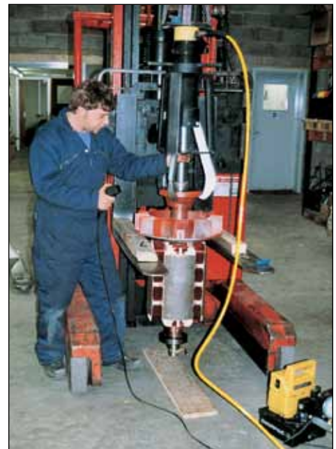
▲ EPH-116 used to remove electric motor pulleys. Puller is positioned using the Lift Plate.
