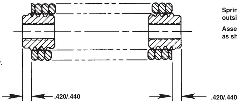
Springs must not extend beyond outside grooves of spring retainer
